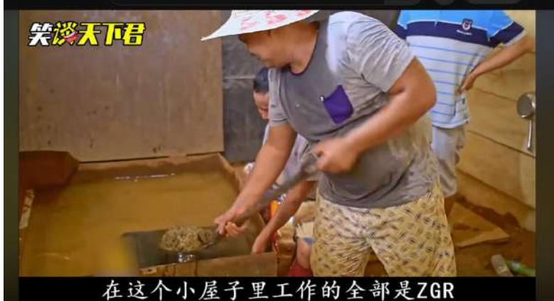
Figure 4 Chinese workers manually washing sediment in a small indoor gold-processing pit to recover gold particles .
